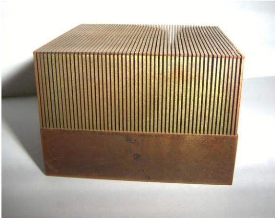
Fig. 1. Bc Cu hair brush – 40 by 40 mm sq. Tines are 21 mm long.
