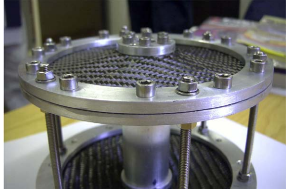
Fig. 2. Carbon cloth support. OD is \sim 135 mm. ID \sim 40 mm.
