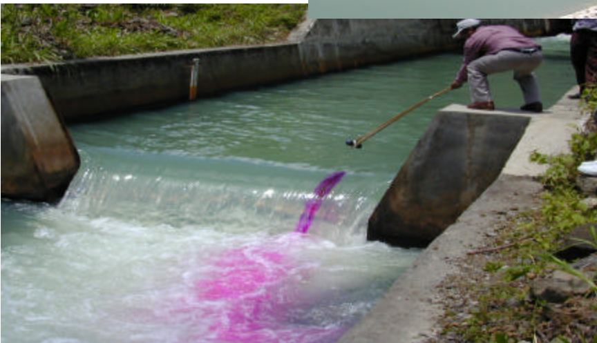
Serma dam, Yogyakarta, Indonesia Discharge gauging with artificial tracers. (Photo credit: E. Garcia-Agudo/ IAEA)
